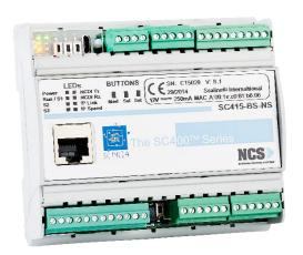
SC4x5™ is a new family of security controllers within the SC400™ range, as part of the SCNET4™ suite from NCS®: integrated electronic systems for managing access control, building security, and technical management. The SC400™ range is suitable for installations in automated, secure buildings and for the most diverse network architectures. It offers great module flexibility, allowing a system to be assembled very economically from building blocks.
