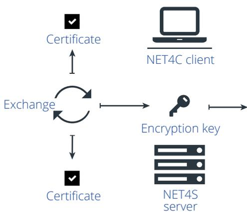
Each SC4x5™ controller contains a web server for configuration and maintenance operations. Access to this web server embedded in the controllers is secured using the HTTPS protocol, which is based on TLS.
